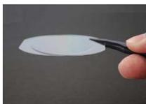
Quartz wafers joined using the atomic diffusion-bonding method
