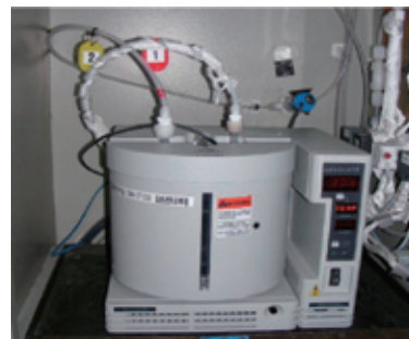
Facility with countermeasures to prevent connection errors
