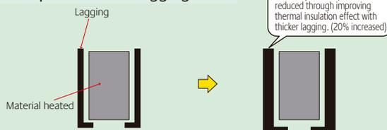
1. Electricity consumption was reduced through improving thermal insulation effect with thicker lagging. (100% implemented)
