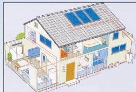
Schematic Diagram of a Solar Water-Heating System
