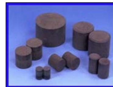
Epoxy molding compound for semiconductor encapsulation
