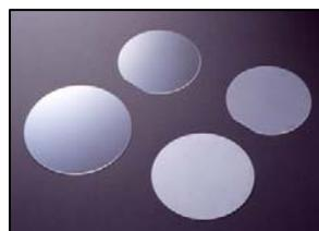
Sapphire substrates for LEDs
