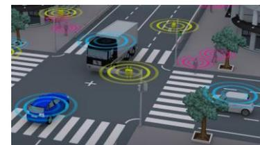
ITS wireless roadside system and far infrared camera technology detect objects in blind spot
